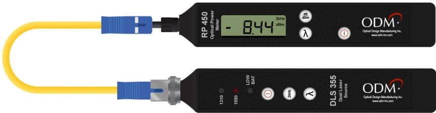
The LFI introduces a bend into the fiber which leaks light from the core onto the detector of the power meter. When using an LFI, expect a 30-35dB offset in core power.
