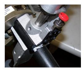
**6.** Repeat the steps 4 and 5 previous. Remove thin chips of insulation and **only drop the blade 2 or 3 revolutions at a time.** Repeat until the conductor is exposed as shown above.
