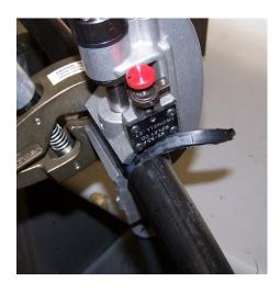
**5.** Turn the tool and engage the blade into the insulation. A small amount of thumb pressure may need to be applied to the thumb knob to cut the insulation. Turn the tool 1 or 2 revolutions to channel out a 3/32" thick chip.
