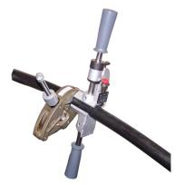
**3.** Lock the tool on the cable, and position it against the stop clamp.
