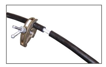
**9.** The stripping process is complete. Remove the tool and the stop clamp.
