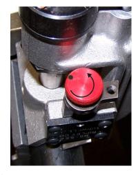
**4.** Turn the red blade adjusting knob 2-3 turns CCW. This will develop a blade depth of approx 3/32". Do not set the blade more than 3 turns. The blade can be damaged by too much insulation removal at one time.
