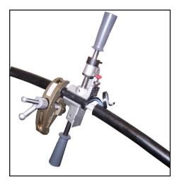
**8.** Apply a small amount of forward pressure and turn the tool to strip the insulation until reaching the stop clamp. Continue turning until the insulation chip breaks away.
