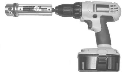
**1.** Insert bushing into tool. Depress the lock collar at the front of the tool, insert the bushing, and rotate it to snap it in place.
