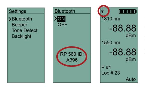
To turn the Bluetooth feature ON, navigate to the Settings menu, select Bluetooth, and Select ON. The RP560 device ID is shown on this screen; take note of it. The Bluetooth icon will be shown on the main screen of the RP560.
