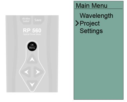
Use the Up/Down arrow buttons to move the cursor to the option you would like to explore. Press the Left arrow button to go back to the Main screen. Press the OK/Menu button or the Right arrow button to select an option.
