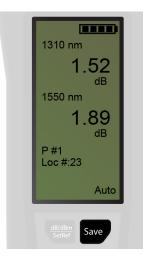
Press the Save button to save both readings.
