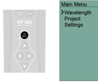
Use the Up/Down arrow buttons to move the cursor to the option you would like to explore. Press the Left arrow button to go back to the Main screen. Press the OK/Menu button or the Right arrow button to select an option.
