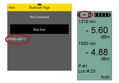
Touch the Scan button, and select your RP560 unit when it appears in the list. When the RP560 is connected to the Android device via Bluetooth, a connection icon will appear on the RP560 screen.
