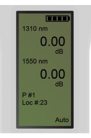
The RP560 will switch to the dB mode for each wavelength, and the readout will display 0.00dB ( $\pm 0.05$ dB).
