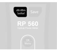
The dBm measurement mode may be used to check the output power of a light source at a specific location in the optical link.
