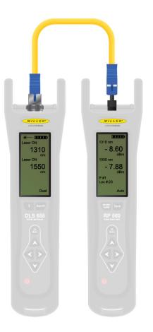
In the example shown here, a DLS 655 dual laser source is being used to set the reference on the RP560 optical power meter. Any singlemode test jumper can be used, provided the adapters on the DLS 655 and RP560 match the connectors on the test jumper.
