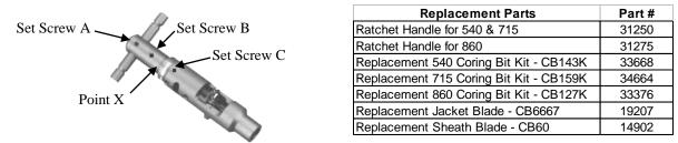
**LUBRICATION**: If tool is purchased with optional ratchet handle, the tool should be lubricated periodically with WD-40 or other light lubricating oil, at Point X.
