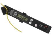
The 2kHz tone output of the DLS 360 can be recognized through the fiber jacket when a Live Fiber Identifier is used.
