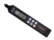
Combine DLS 360 with an optical power meter (RP 460 pictured) to perform insertion loss tests on single-mode fiber.
